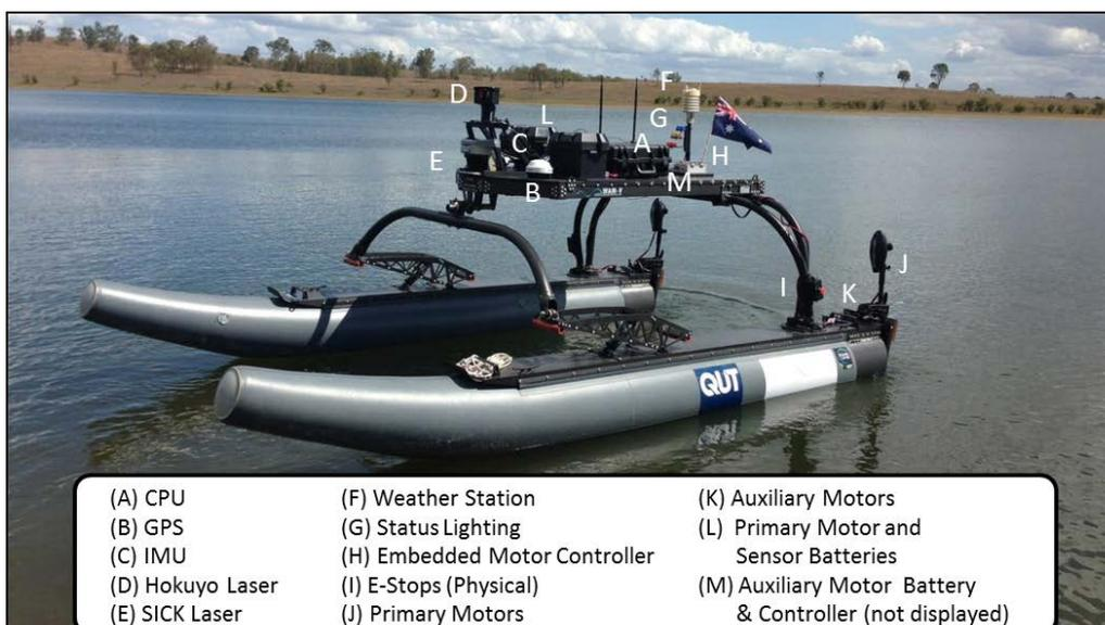
**Figure 1:** The Endeavour ASV showing the location of the sensing, computing, propulsion, safety and power systems (note the hydrophones are not shown but are mounted on motor brackets).
