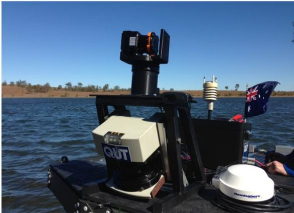
**Figure 2:** Early configuration of the Endeavour ASV sensor suite showing a camera, spinning and nodding laser scanning range finders, GPS, IMU and weather station.
