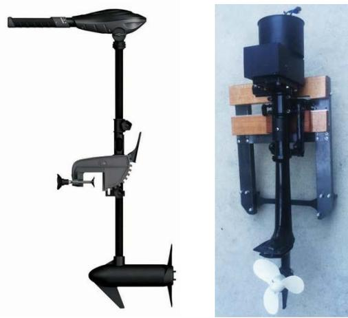
**Figure 3:** The motors used on the Endeavour ASV. (Left) Two Osapian 12V electric trolling motors provide the primary propulsion system. (Right) Custom developed 28.8V electric motors provide a high-speed auxiliary propulsion system (shown attached to the propulsion mounting system).
