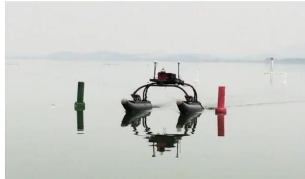
Figure 1 Autonomous Surface Vehicle MACS
