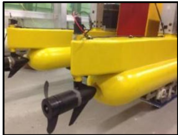
Figure 7. Close-up of Hull-mounted Trolling Motors
