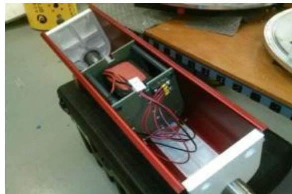
Figure 2. Propulsion Unit under construction
