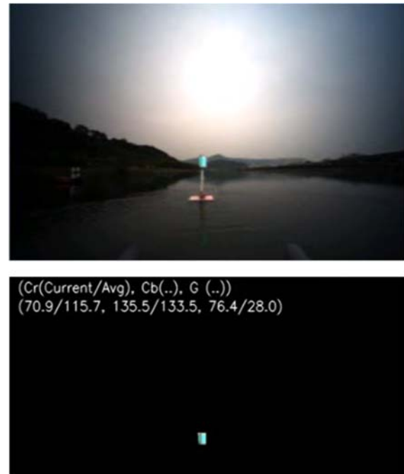
Figure 12. Extracting the LED panel region from the light buoy: camera view (top), extracted ROI (bottom)
