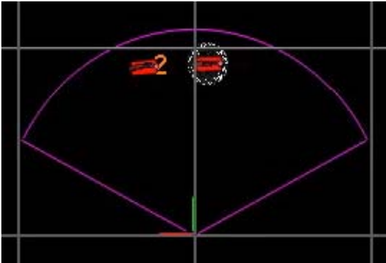
Figure 10. Segmentation and detection of the symbol placards using lidar measurements
