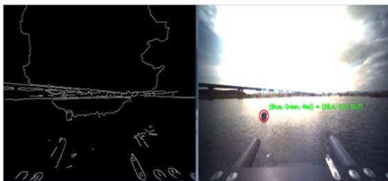
Figure 9. Application of Canny edge detection and Hough transform algorithms to detect the marker buoy
