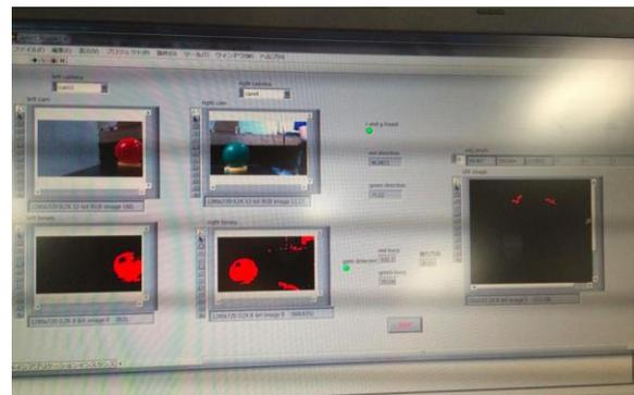
Fig. 11. Color detecting by camera (left) and Object detecting by LRF (Right)
