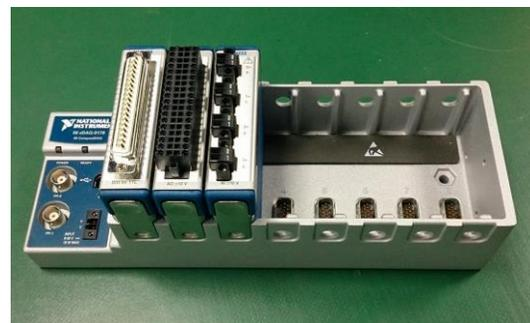
Fig. 6. NI9222, NI9264, and NI9403 installed in c-DAQ9178
